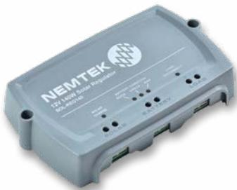
The LED solar regulator offers advanced MPP technology for over 90% efficiency when used with a 140Watt solar panel. It can also be used with solar panels sizes from 20Watt to 200Watts making it very flexible. Larger than the 140Watt solar panels can be used in areas where sunlight intensity is low increasing the capture of sunlight.
