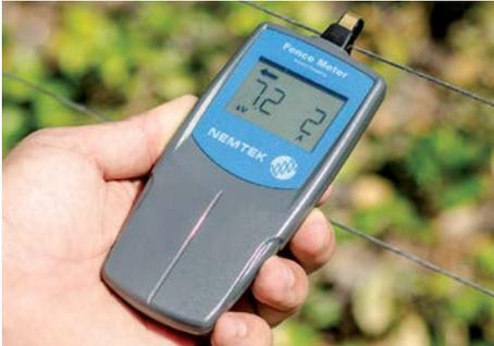
The Nemtek Fence Meter helps diagnose problems on your fence to optimise the electric fence installation and ensure that the fence operates at an ideal level.
