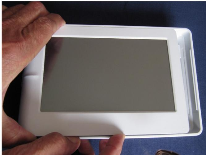
Leverage the LCD out as shown in the picture.
