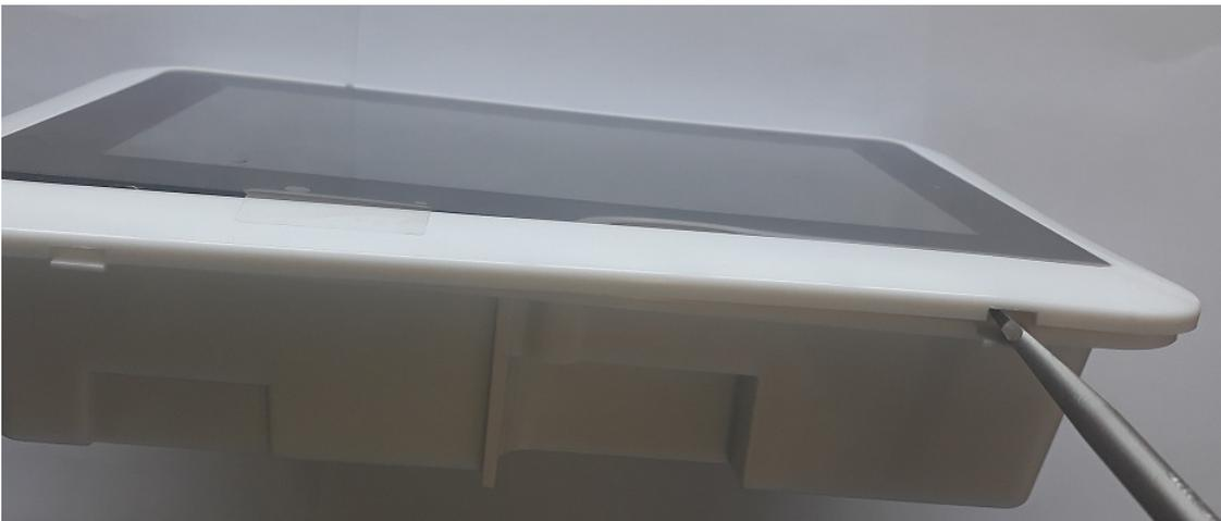
**FG7C CONTROLLER:****OPENING THE FG7C****Wall mount type**
