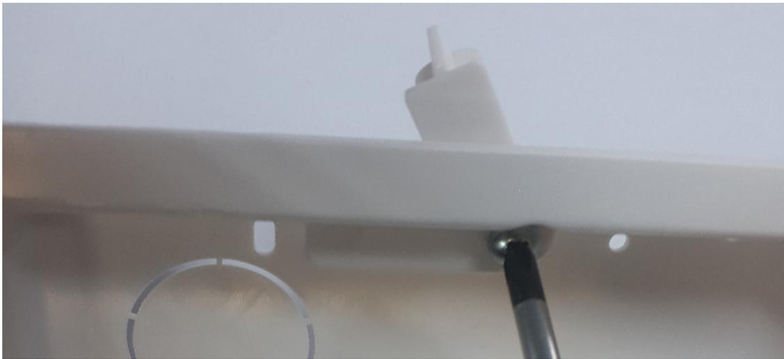
Wing clamp and Wing clamp screw
