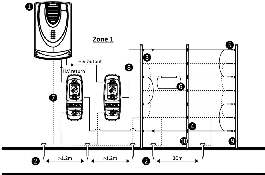
**Installation using a dual zone security energizer**
