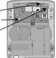
**STEP 6:** Use a drilling template and drill 4 x 8mm holes in the wall for mounting the unit. Four nail-in anchors are supplied with the unit. Insert the plastic sleeve of the nail in anchor into the wall then hammer the screw in with a screwdriver and hammer. **NB: Always insert the plastic sleeve from the inside of the box.**
